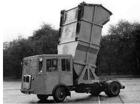
An early 'W' type Fore & Aft tipper tips forwards.
