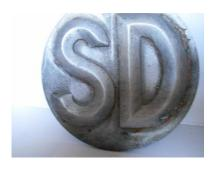
John Oliver from Peterborough has kindly donated the SD radiator badge shown above. It is complete with the fastening bracket on the back. The SD lettering was highly polished when new to give the appearance of chromium plating. This form of badge was used on the 'W' type and also on the Freightlifter fork trucks.
