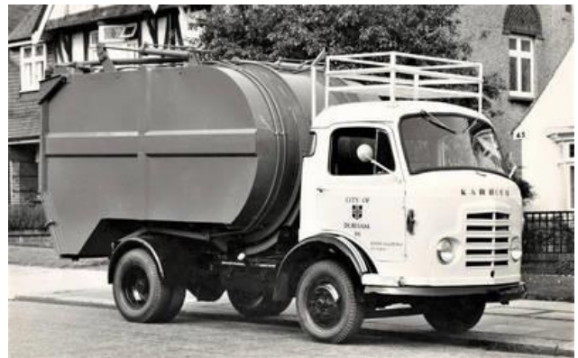
A G.W.& L DualTip on a Karrier chassis.
