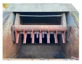
This photo from 4<sup>th</sup> November shows the progress being made on the restoration of the 1974 NY Revopak returned from Malta in 2015 by Aled Rees from Bristol where new tines have been manufactured and welded to the compaction system.
