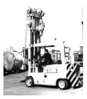
This Defiant 14 is fitted with paper handling equipment and the mast top cable drums can be seen in this photo.
