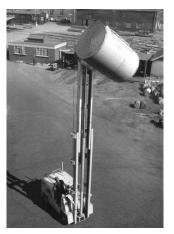
This Model 72 Freightlifter at Reeds' Paper Mill has an outstandingly tall mast for handling paper rolls.
