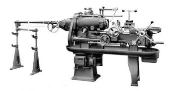
[Your Editor has fond memories of the Ward 2A capstan lathe the first machine he operated at S&D as an apprentice.] When once this was completed I was re-employed as a draughtsman. In 1986 S&D acquired the design, manufacturing and marketing rights of the Cobridge range of road sweepers
