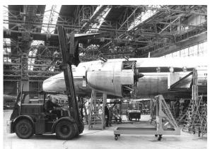
This photo was taken at the Bristol Aeroplane Works at Filton, Bristol, and shows the Freightlifter removing a Proteus Power Plant from the engine stand.
