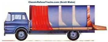
Diagram of the Pak-Mor Mechanism.
