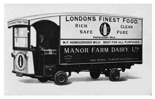
A lovely example of a Freighter for Milk Delivery. 12 ft. x 5 ft. 9 ins. x 6 ft. 6 ins. Load 2 Tons..
