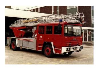
Paul Warnock sent in this photo of an SD WY Turn table ladder YVN 67 Y that was based at Harrogate fire station with North Yorkshire fire and rescue. The ladders were transferred from an AEC appliance and fitted to the SD cab and chassis. On seeing this photo Ronnie Farrington wrote:- "I remember that a turntable ladder came to Manchester S D depot. I think gear box problems were discovered on a pre delivery inspection."
