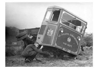
From the driver's point of view the mishap to St. Helen's gas department Freighter was less serious. It demonstrates, I believe, the dangers of driving on landfill sites as the ground appears to have given way under this Freighter. A second photo gives more detail of the damage caused.
