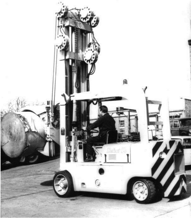
A further picture of a DT12 with brick handling equipment.
