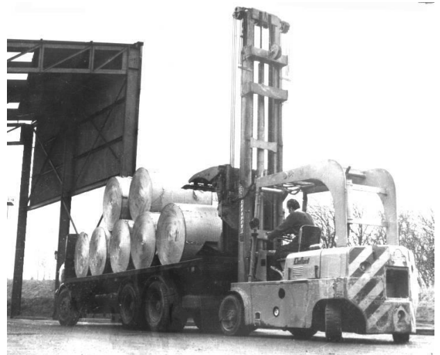
This DT14 equipped for paper handling has a tilt frame fitted because of the extra lifting height provided.
