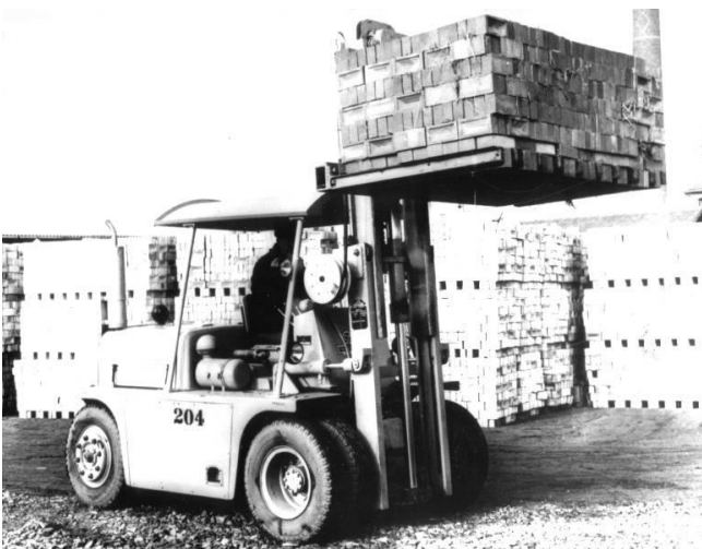
This DT14 equipped for paper handling has a tilt frame fitted because of the extra lifting height provided.
