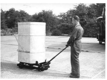
Here a Paladin container is lifted on the hand trolley ready to be fitted to the rear of the vehicle for discharge.
