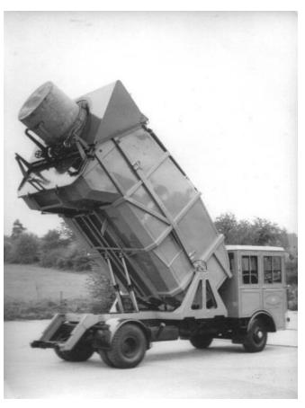
As the Fore & Aft body is tipped forward the contents of the container are discharged into the body.
