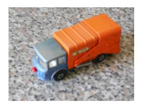
Recently I came across this version of the SD 'T' series Pakamatic Matchbox model with its curious protrusion from the radiator grille. Turning the socket headed screw raises the body as if tipping to discharge the refuse. It operates via a worm and wheel situated by the back axle. I wonder how many of this model were produced by Matchbox?
