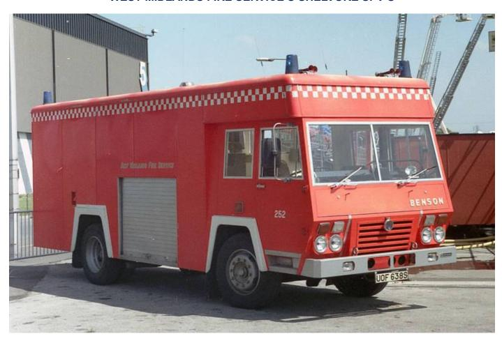
The above photo of a Shelvoke SPV Fire Appliance delivered to the West Midlands Fire Service as a Mobile Control Unit in 1977 carries bodywork by Carmichaels of Worcester using a 'Benson' cab and with the registration number **UOF 638 S**.
