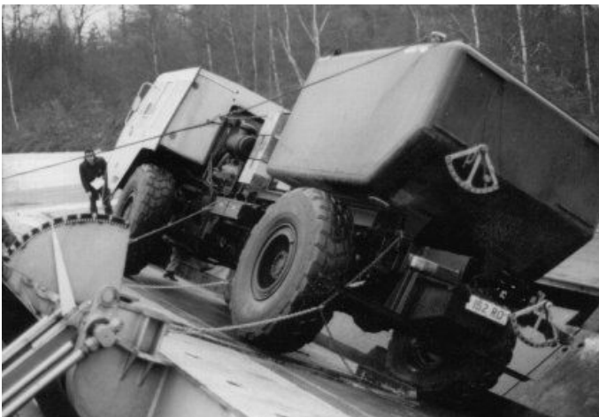
A Crash Tender chassis on the tilt test at Chobham.
