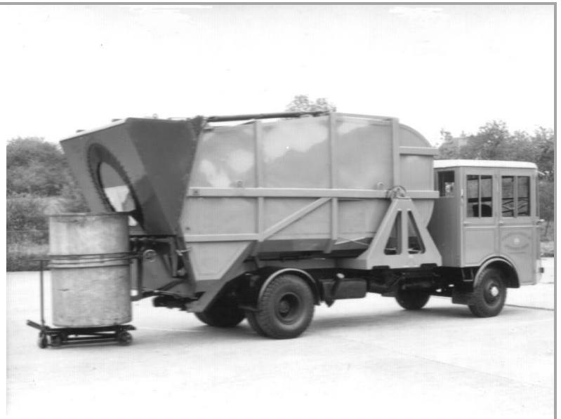
Above :- The Palladin container was popular for commercial premises, flats and apartments. The revision to the SD 'W' type Fore & Aft tipper permitted waste from bulk containers to be collected by the vehicle.
