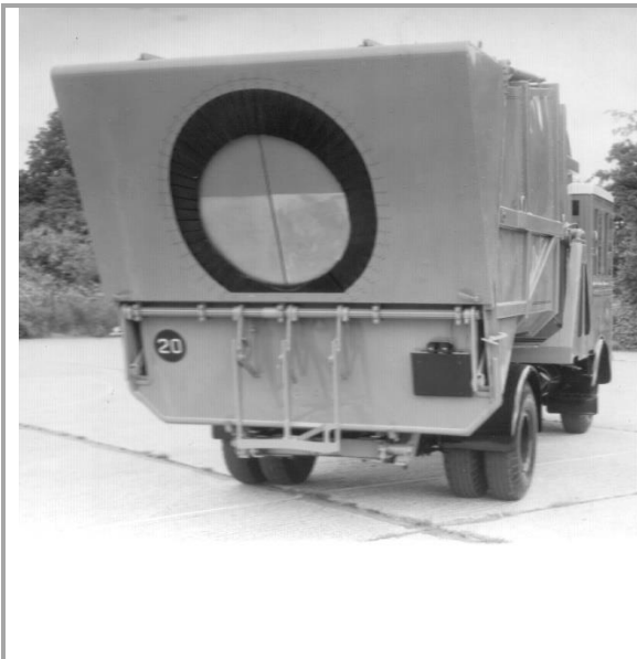
Above :- In 1953 a modified rear door and bin lifting equipment allowed the Fore & Aft tipper to handle bulk waste.
