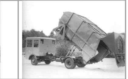
Above :- The Palladin container was popular for commercial premises, flats and apartments. The revision to the SD 'W' type Fore & Aft tipper permitted waste from bulk containers to be collected by the vehicle.
