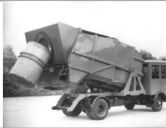
Above :- The Palladin container was popular for commercial premises, flats and apartments. The revision to the SD 'W' type Fore & Aft tipper permitted waste from bulk containers to be collected by the vehicle.
