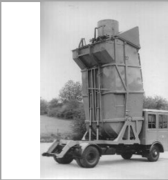
Above :- The Palladin container was popular for commercial premises, flats and apartments. The revision to the SD 'W' type Fore & Aft tipper permitted waste from bulk containers to be collected by the vehicle.
