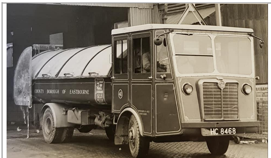
In 1947 the new 'W' type was launched, with conventional steering wheel and gearbox.
