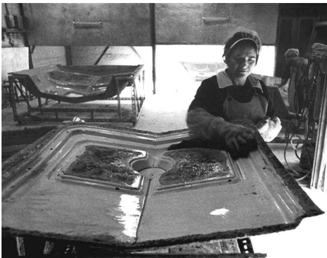
Above:- Another photo by Bill Smith shows a fibreglass radiator cover under construction.
