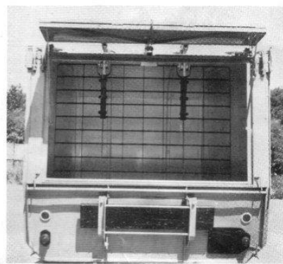
Above :- The Power Press plate in the lowered position.
