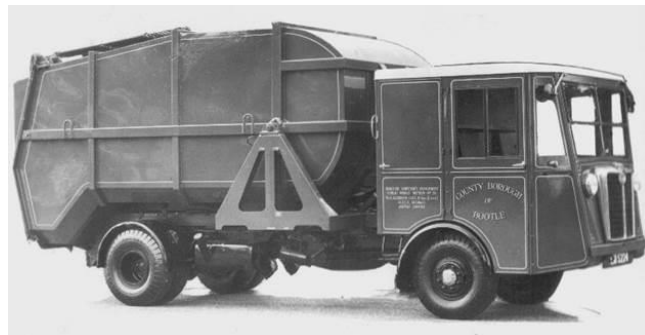
A typical 1950’s SD vehicle – the ‘W’ type Fore & Aft tipper.
