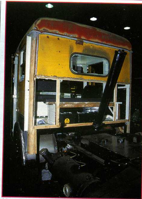
Note the new ash framing in the cab.
