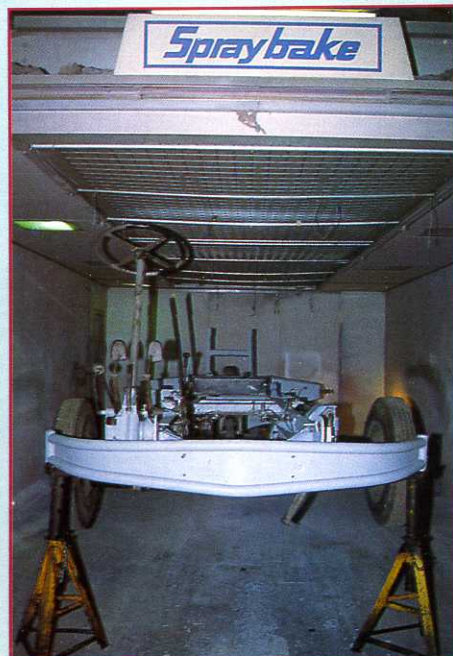
The chassis propped up on axle stands in the oven prior to the preparation and paint work commencing at Hatfields Motors. Notice the wheels turned inside out - this gave Frank the painter easier access to the chassis.
