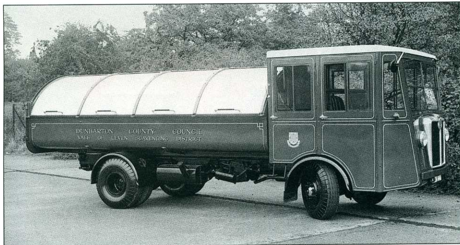
1953 W-type with conventional side loading dustcart bodywork.
