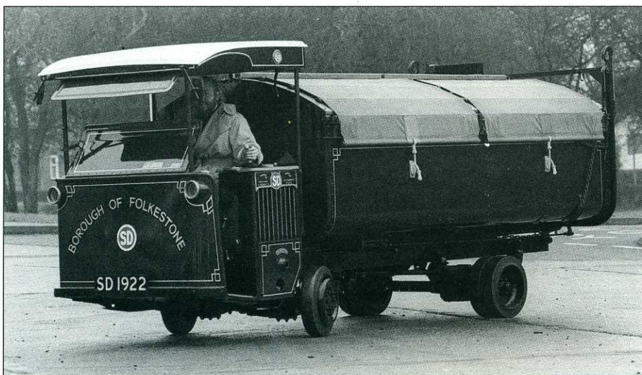
Nick Baldwin tries the tiller controls of the early Freighter that S&D restored to resemble their first vehicle of 1922.
