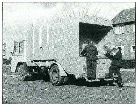
Loading a 1973 Pakamatic on a S&D chassis but also available on proprietary types.
