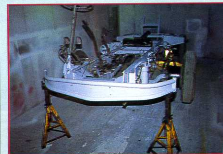
The chassis just prior to the start of the painting.
