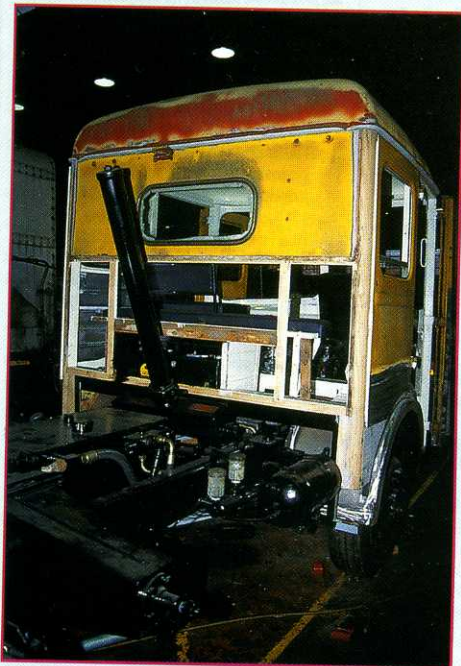
The cab is now reunited with the chassis and the S&D begins to take shape once more. Note the fine workmanship evident on the chassis.
