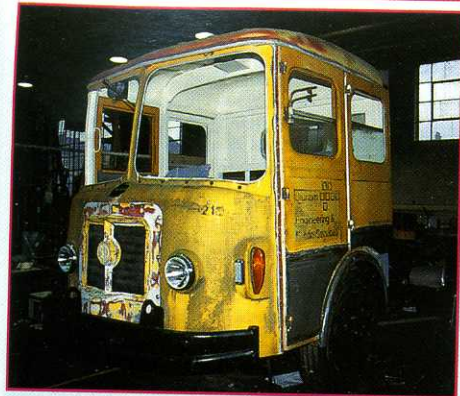
These two shots show the cab from the near and off sides, with the new sections visible in the lower doors.
