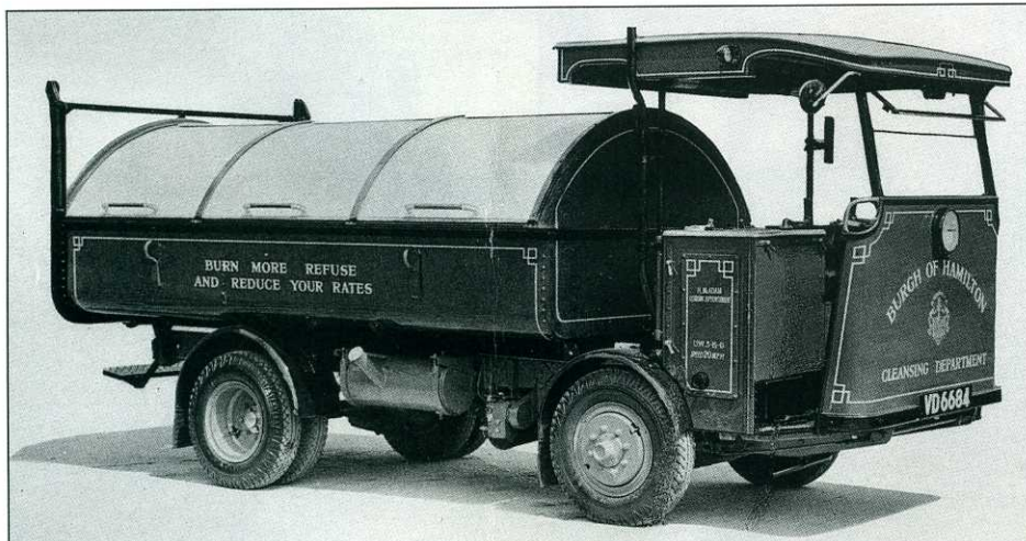
One of the late tiller steered tipper from 1936. This one for Hamilton had a demountable body.
