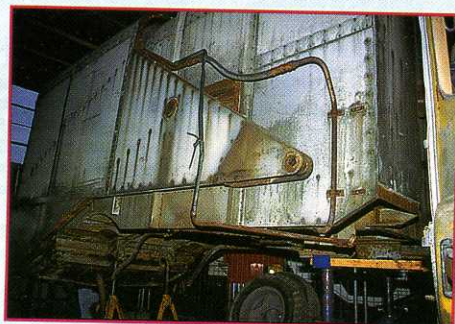
A view of the body propped up on axle stands awaiting repairs.
