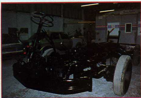
Transformed! The chassis after repainting and baking. There is a lovely gloss finish to the paintwork - well done Frank!
