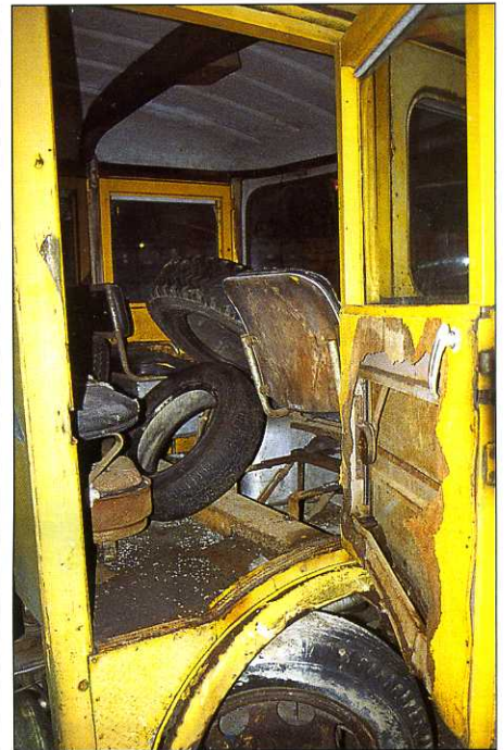
The rear door compartment which was used by the dust men has had the door panel ripped off and the spare tyre certainly does not fit this lorry.
