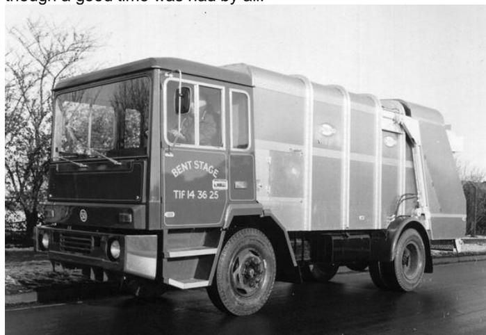
This interesting photo shows a PN Revopak equipped with a wooden mock up cab to test out the ability to produce a left hand drive version for Bent Stage in Denmark.
