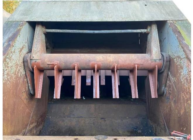
This photo from 4<sup>th</sup> November shows the progress being made on the restoration of the 1974 NY Revopak returned from Malta in 2015 by Aled Rees from Bristol where new tines have been manufactured and welded to the compaction system.
