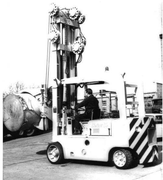
**This Defiant 14 is fitted with paper handling equipment and the mast top cable drums can be seen in this photo.**
