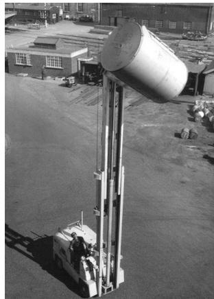
This Model 72 Freightlifter at Reeds' Paper Mill has an outstandingly tall mast for handling paper rolls.
