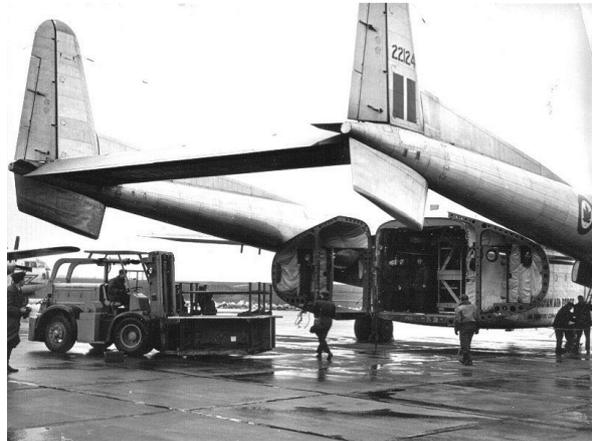
I believe the above photo was taken at RAF Wittering (It was taken by the Stamford Mercury) but it appears to be a Canadian aeroplane. (Roger identifies this as a R.C.A.F. C 82 Fairchild Packet.) Note the non-telescopic mast on the Model 82 Freightlifter.
