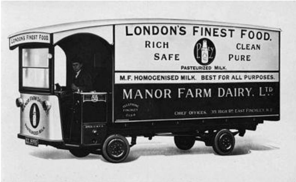
A lovely example of a Freighter for Milk Delivery. 12 ft. x 5 ft. 9 ins. x 6 ft. 6 ins. Load 2 Tons..
