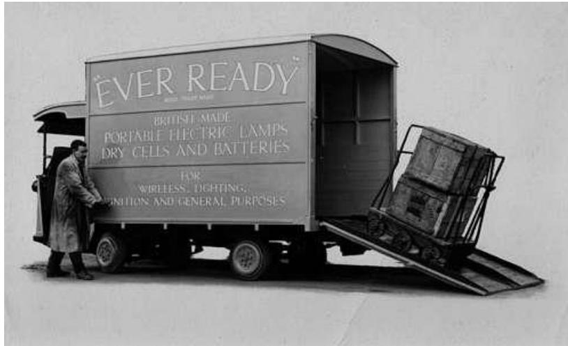
BOX VAN WITH WINCHES AND RAMP END. 10 ft. x 6 ft. 6ins. LOAD 2 tons. Price £640
