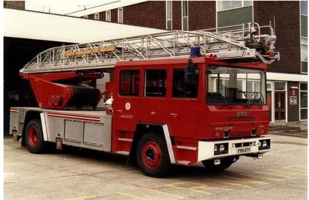
Paul Warnock sent in this photo of an SD WY Turn table ladder **YVN 67 Y** that was based at Harrogate fire station with North Yorkshire fire and rescue. The ladders were transferred from an AEC appliance and fitted to the SD cab and chassis. On seeing this photo Ronnie Farrington wrote:- "I remember that a turntable ladder came to Manchester S D depot. I think gear box problems were discovered on a pre delivery inspection."
